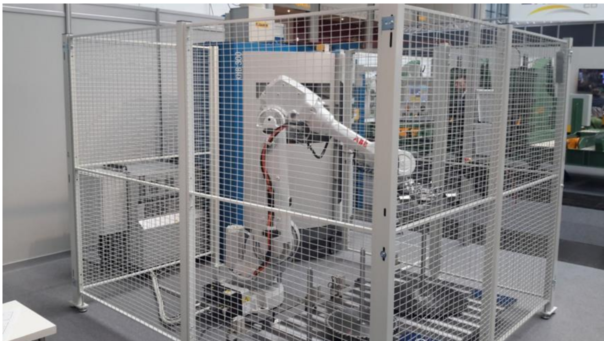
Figure 1. An automated robotic arm inside a factory workcell. The robot is within a cage to ensure the safety of humans in the vicinity.
