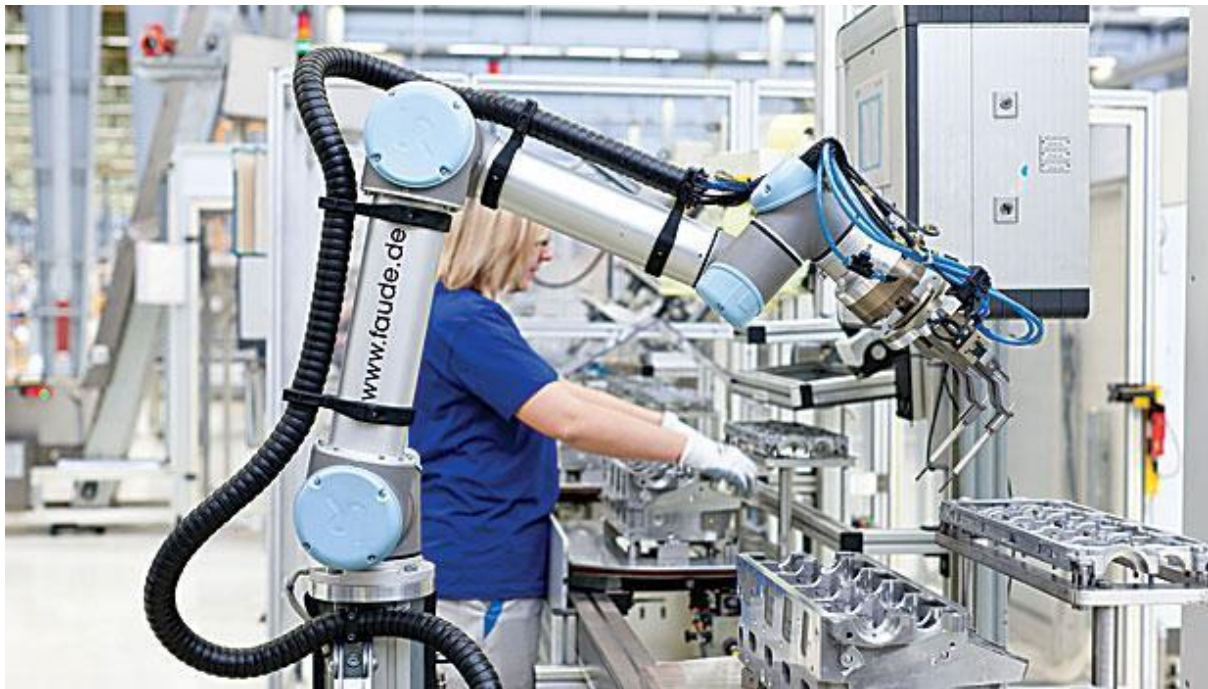
Figure 3. A collaborative robotic arm that can safely work alongside humans.
